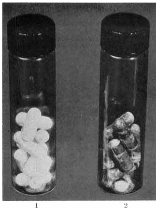
Fig. 1.—1, Capsules of pyrilamine resin adsorbate, aspirin, and sodium ascorbate; 2, Capsules of pyrilamine maleate, aspirin, and sodium ascorbate, after 1 month of storage at 45°.
